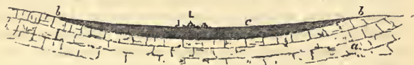
FIG. 49.—Section to the position of the water-bearing rocks below the clay at London.
